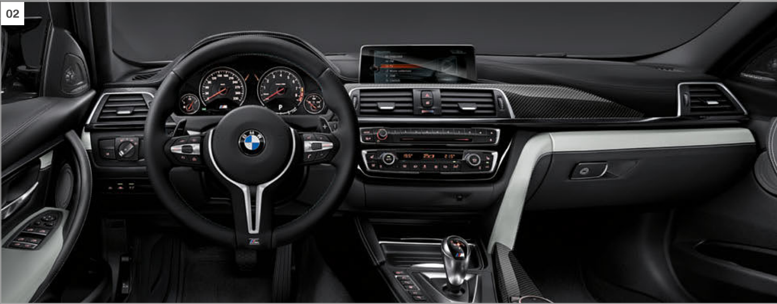
[ 01 ] The bold design demonstrates the innate power of the BMW M3 Saloon. [ 02 ] The athletic interior is characterised by typical M driver orientation and perfectly crafted materials. The ergonomically optimised gearshift lever of the optional Seven-speed M Double Clutch Transmission (M DCT) with Drivelogic conveys motorsport feel and the free-standing Control Display screen presents all options in absolute clarity.
